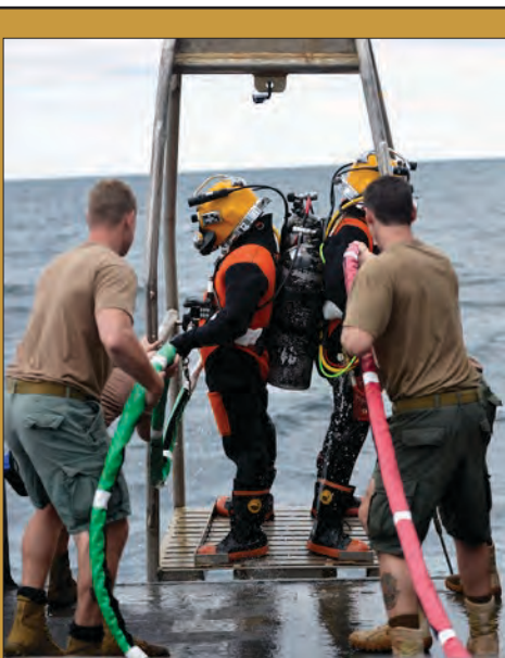
Divers clear the side of the ship and are lowered on the diving stage into the water during air surface supplied diving operations off the coast of Virginia. Navy Divers performed deep-sea salvage operations aboard the rescue and salvage ship USNS GRASP (T-ARS 51) to recover the wreckage.
